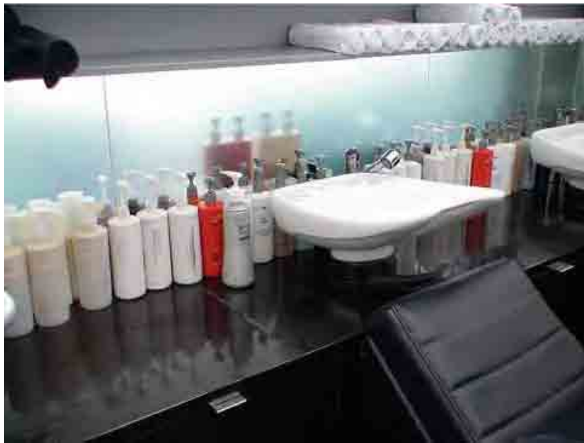
Figure 3: Figure 3. Difficult side access to the basin – Undesirable.
